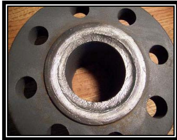
Figure 6. Crevice Corrosion at the ID of the flange
