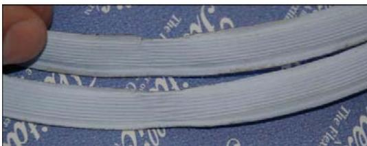
3.4 Test 4 The underside surface of the gasket was removed and examined for damage after each compression test, the core was refaced before the sealing test.
