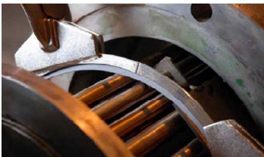
The core is aligned using wide jaw clamps and supporting sacrificial backing rings, these are stainless rings which are sized as the sealing element. This backing ring provides support for
