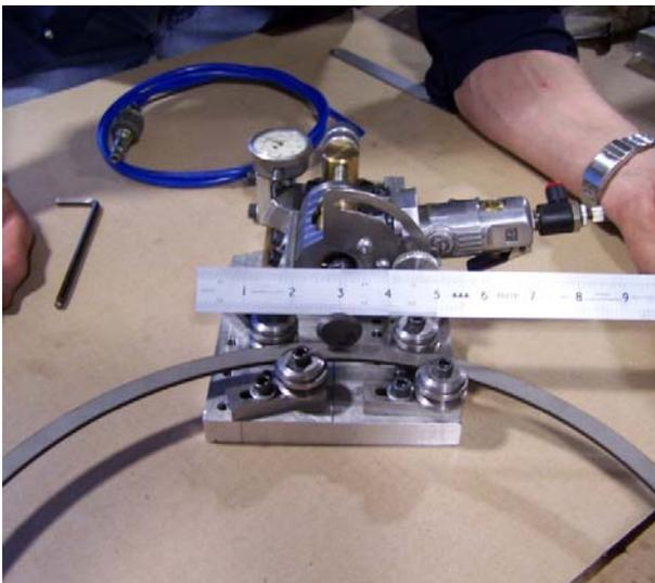
After the initial groove is re-machined, the cutting tool is raised to a level sufficient to clear the surface of the ring. The cutting tool is then indexed inward based upon the factory machining specifications of the ring. Alternately, the same procedure used to set the initial groove location may be used.
