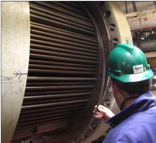
Site inspection of previously used shell to tubesheet gasket
