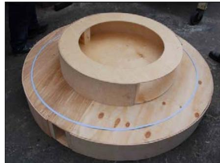
Full scale wooden model of the heat exchanger showing gasket position
