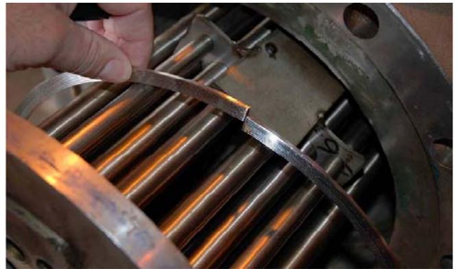
environment. A purpose designed compressed tool was developed. The serration depth, spacing is key to a successful seal. Groove alignment is achieved from clamping the rings prior to welding. Groove depth and spacing is determined by the tool, using a cam machined in the bush depth is controlled, spacing determined using a micrometer.
