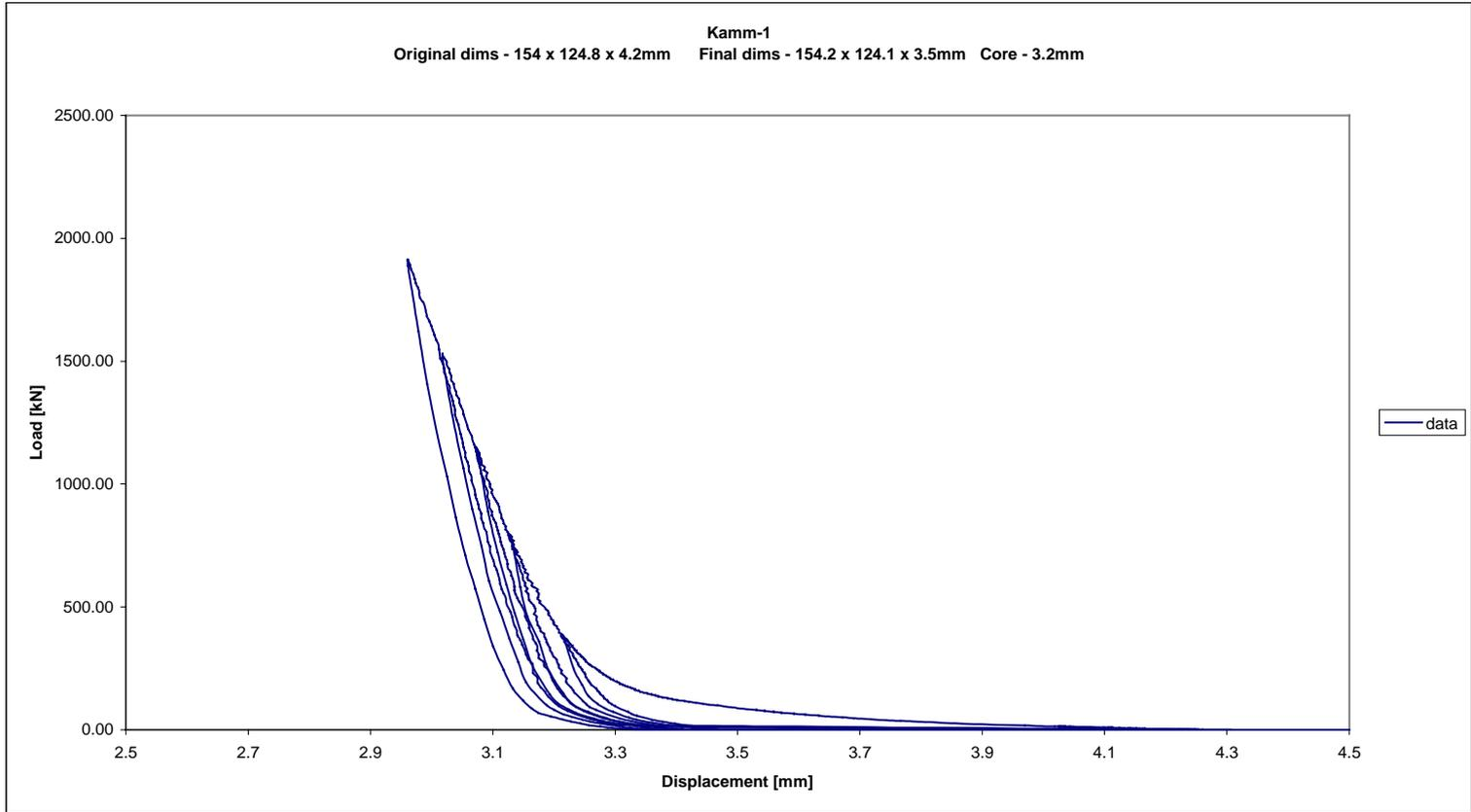
Fig 2.5 Load v Deflection of Serrated Core with Graphite Facing
