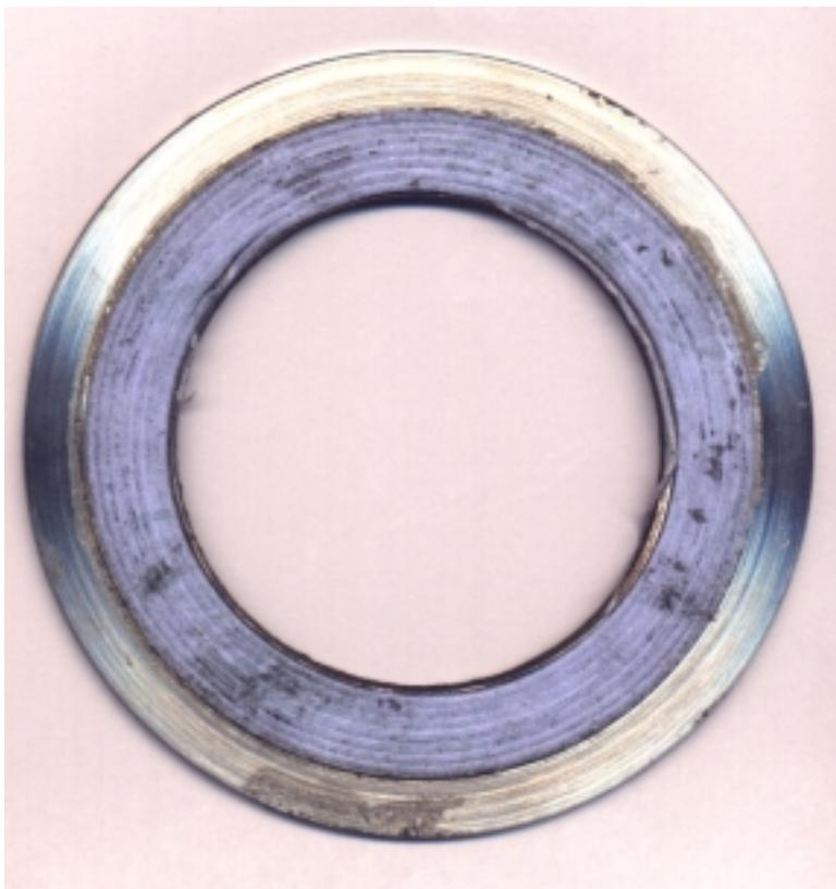
Fig 2.8 Serrated Metallic Core ptfе Faced after Compression
