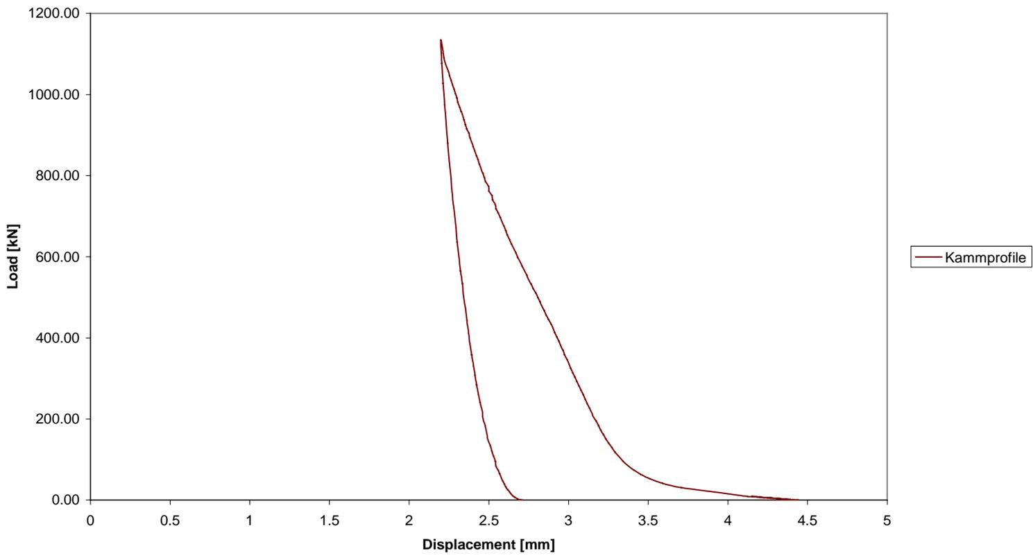
Fig2.6. Load v Deflection for ptfе Faced Serrated Core
