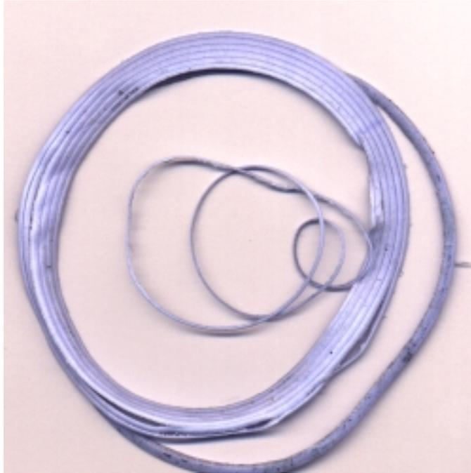
Fig 2.9 ptfе facing removed from Serrated Core after Compression
