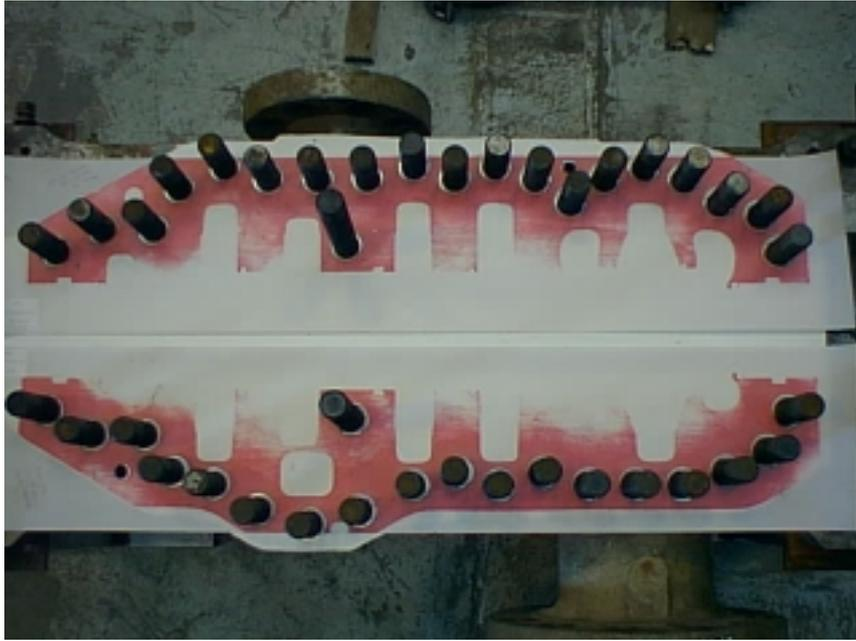
Fig. 1.2 Typical Compression Pattern on Stress Sensitive Film
