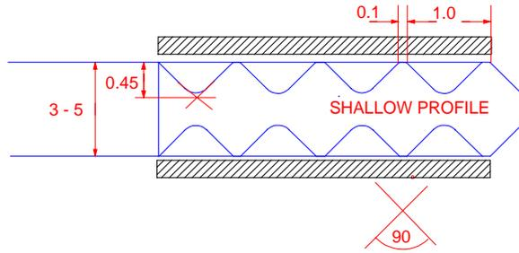
Fig2.4 Section Serrated Metal Core with Facing
