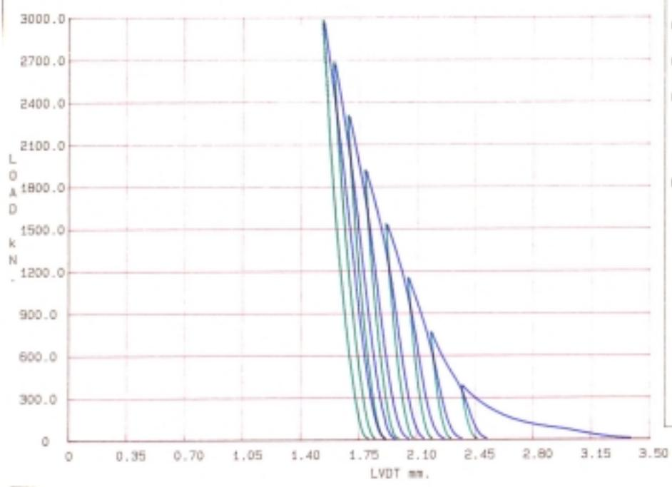
Fig2.2 Load Deflection Curve for Jacketed Gasket
