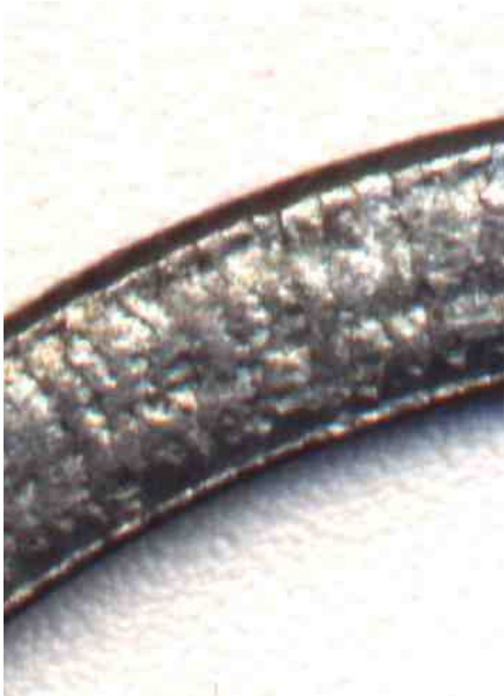
Fig 3 , Magnified Image of metal washer, Header side, showing machine marks on header flange.
