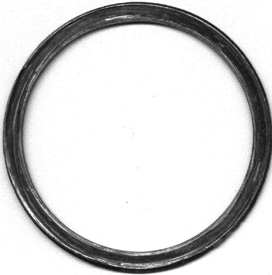
Fig 1, Solid metal washer, showing scratch marks from metal plug.
